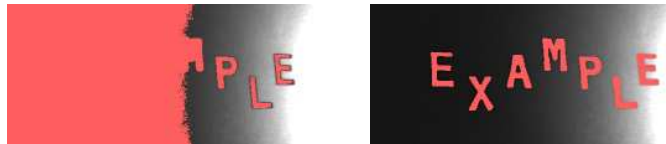
Results of ThresholdToRegion and ThresholdToRegion_Dynamic on images with uneven light.
