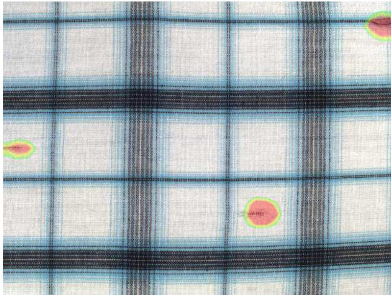
An example of textile defect detection using the FisFilter_DL_DetectAnomalies2 .
