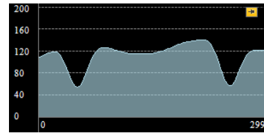
Too high inSmoothingStdDev - significant edges are attenuated
